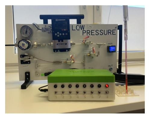
Figure S2. Photo of the up to 10 bar pH<sub>2</sub> bubbling setup, which scheme and rendering are shown in Fig S1. The video of the system performance is available as an additional video file.
