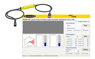
The User Configuration Tool (UCT) offers an easy way to link I/O points in your wireless network, view I/O register values graphically, and set system communication parameters when a host system is not part of the wireless network.
