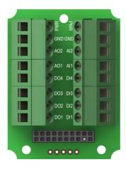
Alx or Ax. Analog IN x. AOx. Analog OUT x. DIx. Discrete IN x. DOx. Discrete OUT x. GND. Ground/dc common connection. PWR. Power, 10 to 30V dc power connection.
