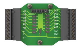
Alx or Ax. Analog IN x. AOx. Analog OUT x. DIx. Discrete IN x. DOx. Discrete OUT x. PWR. Power, 10 to 30V dc power connection. RX/-. Serial comms line TX/+. Serial comms line V+. Power, 10 to 30V dc power connection. V-. Ground/dc common connection.
