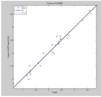
Figure 3: Predicted surface roughness against the actual surface roughness
