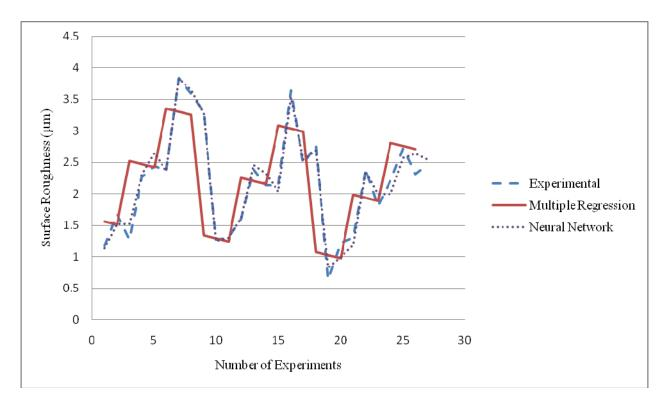
Figure 4: Plot of predicted using multiple regression and neural network and actual experimental surface roughness
