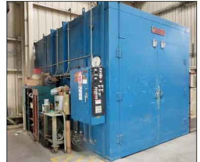
Wisconsin Model EUN-814-8G Natural Gas Fired Drive-In Cure Oven
