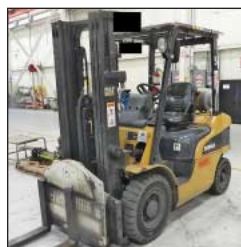
(4 or 5) Various Lift Trucks, Most Likely 5,000 Lb. Caterpillar Model P5000 LP Gas Lift Trucks
