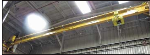
(10) 1 Ton to 5 Ton x 35' to 55' Span Single Girder Top Running Overhead Bridge Cranes
