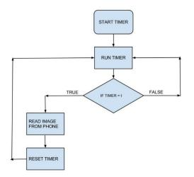
Figure 5 MATLAB function for reading transmitted video.
