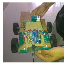
Figure 10 A picture of the robot, with the Arduino on top
