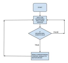
Figure 9 Flowchart depicting functioning of Arduino
