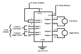
Figure 8 A circuit diagram of the motor driver circuit
