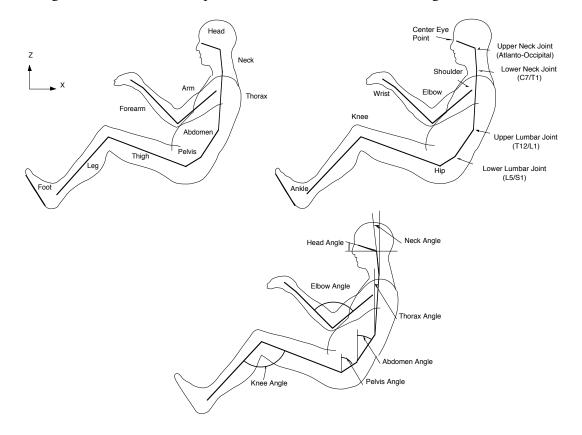
Figure 6. Definitions of kinematic linkage and posture measures (Reed et al. 1999b). Angles referenced to horizontal or vertical are XZ (sagittal) plane angles. Angles between segments (elbow angle, knee angle, and ankle angle) are measured in the plane formed by the segments (included angles). Note: Neck angle is negative as shown. All other angles are positive as shown.
