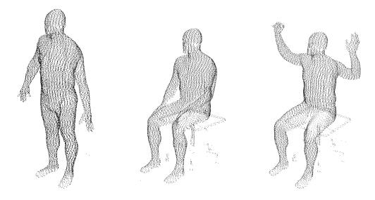
Figure 4. Postures used for CAESAR scans (from top, A, B, and C), shown as point cloud data (approximately one tenth of data points are shown).
