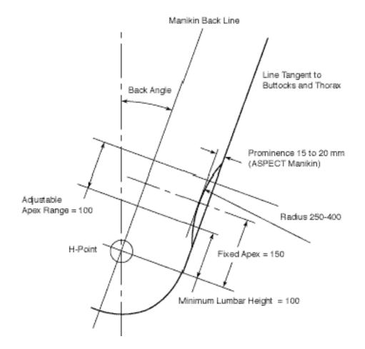
Figure 9. Schematic illustration of lumbar support recommendations (dimensions in mm).
