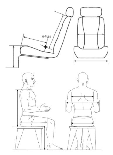
Figure 1. Seat dimensions (top) and related standard anthropometric dimensions (bottom).
