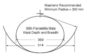
Figure 3. Illustration of compatibility between Maertens' (1993) lateral backrest contour specification for 250 mm above the depressed seat surface and 95th-percentile-male waist dimensions. Waist cross-section is shown as an ellipse--actual body shape is flatter toward the rear, which may affect the fit between the seat cross section and sitter's back.
