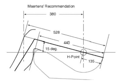
Figure 2. Comparison of Maertens' (1993) and current recommendations for maximum cushion length. (Dimensions in mm -- see text for explanation.)
