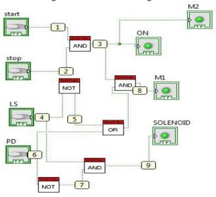
Fig.12. Block Diagram View of Automatic Bottle Filling System
