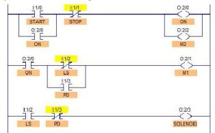
Fig.9. Ladder Diagram for Automatic Bottle Filling System
