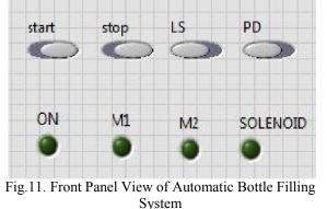
The input to the system is given through switches and output is displayed using LED. Fig. 11 shows the front panel view of the automatic bottle filling system in LabVIEW. The block diagram view of the same system is as shown in Fig. 12 with reference to Fig. 9.
