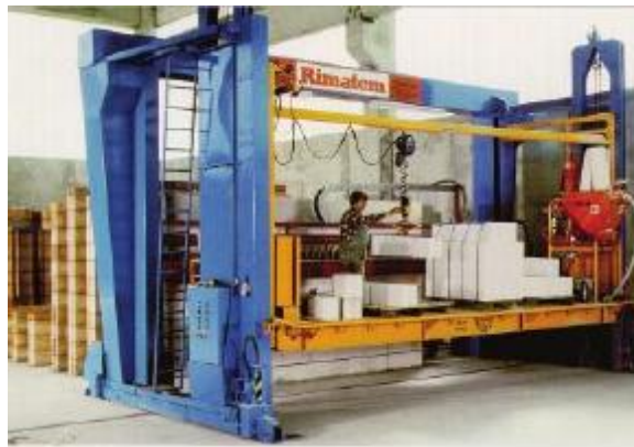
Figure 9. Factory-based mobile semi-automated masonry wall production unit including automated mortar distribution, [Bock 2008].
