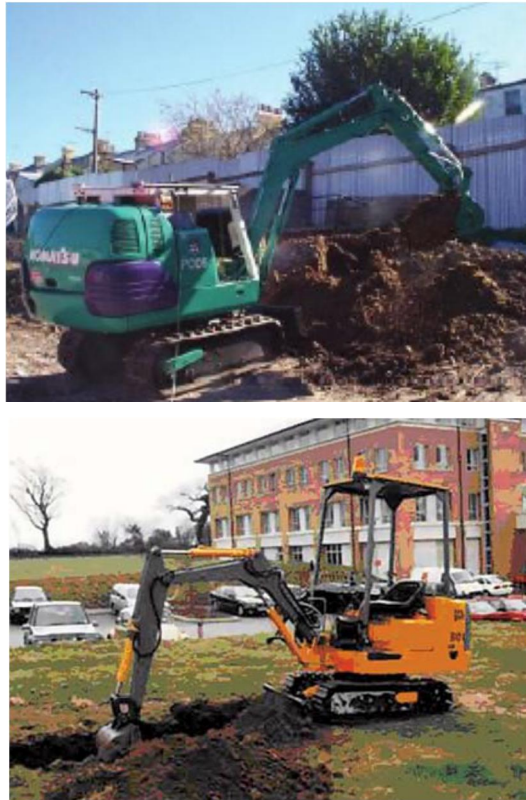
Figure 10. Automated excavator from the University of Sidney [source: Balaguer & Abderrahim 2008] and LUCIE -Autonomous excavator [source: Saidi et al. 2008].
