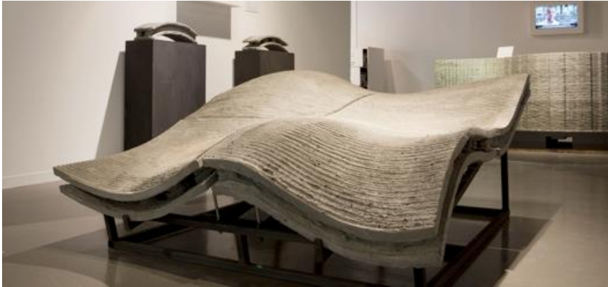
Figure 20. Reinforced concrete element manufactured using 3D concrete printing. [ http://www.buildfreeform.com/ ]
