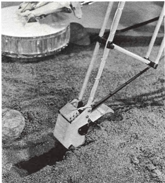
Figure 2. Simulated Lunar Trenching Operation - SM/SS
