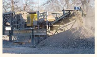
Fig. 9 Crushed concrete from other sources can serve as recycled aggregate. Photo: Portland Cement Association.
