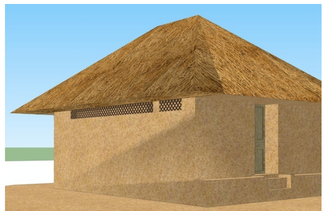
Fig. 15. Extended Eave projection and bamboo meshing to prevent rain ingress and allow ventilation
