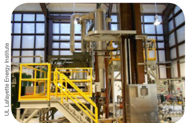
3-Ton/day Biomass fed gasifier processes wood chips to generate power and fuel. (Cleco Alternative Energy Center)
