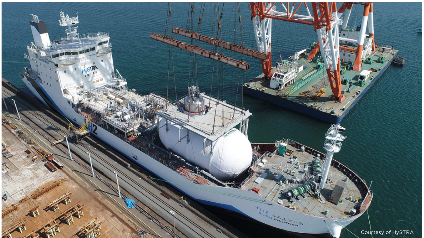
Figure 15: The Suiso Frontier is the First Liquid Hydrogen Carrier, Launched in 2019 and Intended for Use in the HESC Pilot Project
