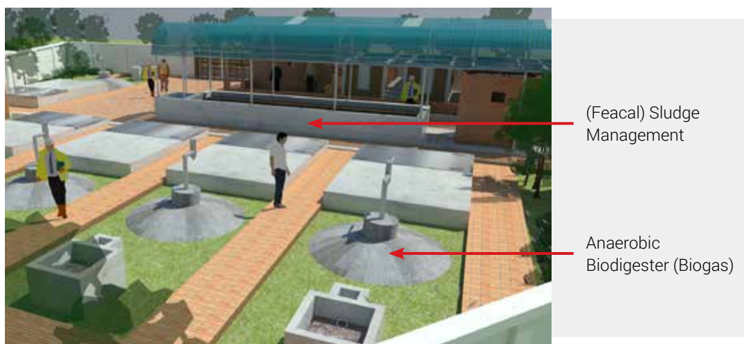
Figure 3.c. Isometric view of IRRC in Malang Regency, Indonesia (with compost plant, biogas plant, faecal sludge treatment plant, and trickling filter for waste water treatment plant).
