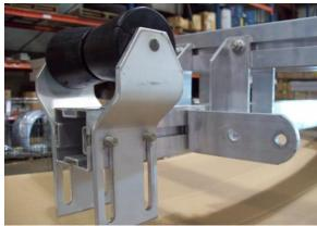
Slide the bolts into the slots on the side of the rear tongue section.
