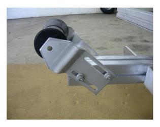
Angle the rear roll as shown and tighten all nuts.
