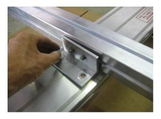
Re-install the cross member attaching angle that was removed previously.
