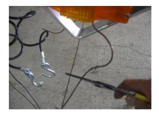
Cut 6" off of the brown wire on the left (driver's side) running light. <u>Do not strip the wire.</u>
