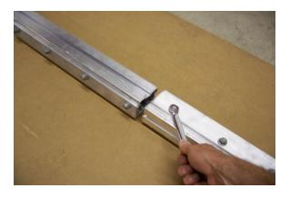
Loosen eight nuts on each splice plate.
