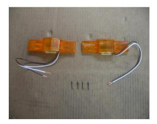
Locate the two amber running lights and four small Philips screws.
