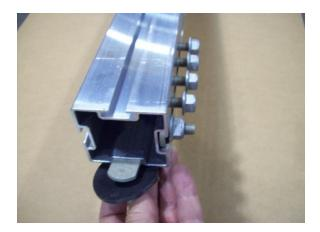
Locate the 1 1/8" T-bolt that was previously removed. Put it into the bottom slot at the back of the rear tongue section, slide it forward approximately 62" and leave it there.
