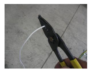
Cut the white ground wire at the front of the trailer leaving it 22" long. Strip the wire and install a ring terminal as previously described.
