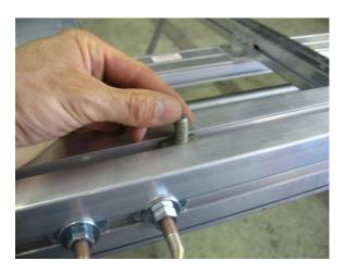
Slide the ¾" T-bolts on either side of the 1 1/8" T-bolt. At this point you should refer to the Hobie Cat instructions for installation of the cradles.
