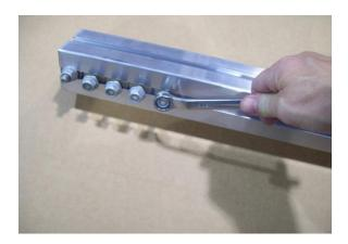
Remove the nuts from the forward most bolts located on either side of the back of the rear tongue section.
