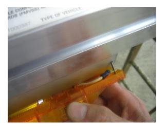
Install the running lights into the pre-drilled holes in the running light bracket using a Philips screwdriver. Be sure the screw is through the ring terminal on the back side of the lights. This will supply a ground to the lights. <u>DO NOT OVER TIGHTEN.</u>
