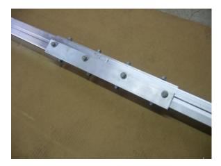
Slide the other splice plate onto the adjacent tongue section. Tighten all 16 nuts making sure that the tongue sections are as tight as possible to one another.
