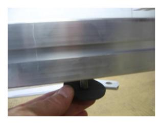
Install the rubber washer that was removed previously onto the 1 1/8" T-bolt located in the bottom slot approximately 62" from the rear
