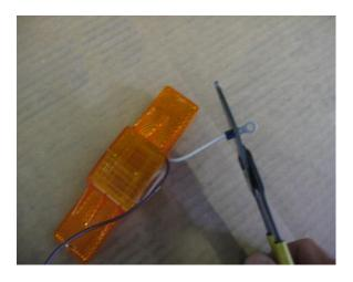
Install the ring terminals by crimping the terminal onto the bare wire.
