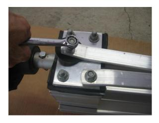
Remove the  $1\ 1/8$ " T-bolt and rubber washer located on the tie rod end and set them aside for installation later.
