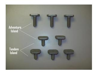
Locate the (3) 1 1/8" and (2) 3/4" T-bolts (used for Adventure Island). Locate the (5) 3/4" T-bolts (used for Tandem Island).
