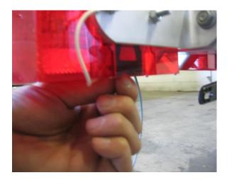
Locate the black tab at the bottom of the right (passenger side) tail light.
