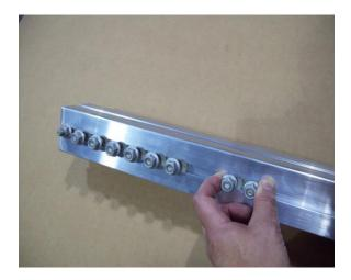
Loosen the two forward most T-bolts (two on each side) located at the end of the rear tongue section.
