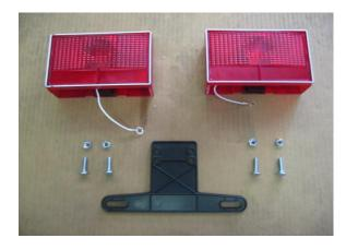
Locate the tail lights, carriage bolts, and nuts inside the light kit box.
