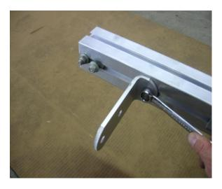
Install the tail light brackets loosely and slide them toward the front of the trailer - final location to be determined later.
