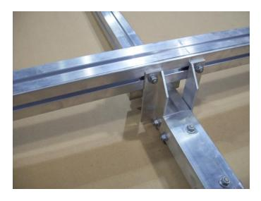
Attach the cradle bracket to the tongue section aligning the angles with the pencil marks on either side of the tongue section. Align the angles with the pencil marks on the cradle holder. The cradle holder bracket should rest against the tongue splice plate as shown.
