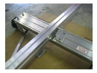
Attach the tongue section to the axle assembly with the tie rods facing forward.
