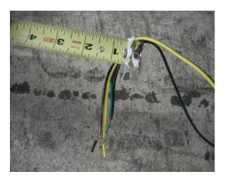
Attach both wires of the harness to the end of the tape measure using the ties provided with the harness.
