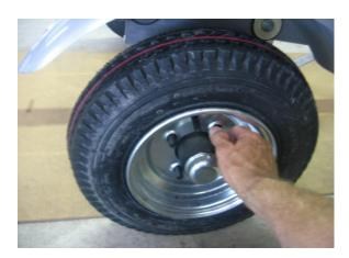
Install the wheels with the valve stems facing out. Install the lug nuts with the tapered side facing the wheel. Tighten to 80 foot pounds in a crossing pattern. Re-tighten after 25 miles.
