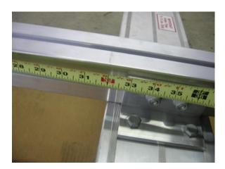
Align the rear edge of the axles assembly with the pencil line on the bottom of the tongue section located at 32" from the rear.
