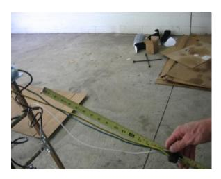
Pull the excess wire out of the back of the tongue section leaving approximately 18" of harness exposed at the front.
