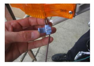
Pass the brown wire from the other running light through the remaining open slot in the connector at a point close to the running lights.
