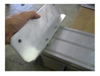
Install the fender brackets onto the bolts.
