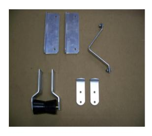
Roll assembly, skid, tail light brackets, fender brackets.
