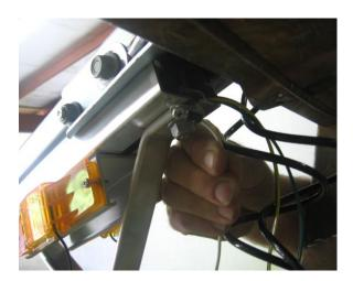
Install the ground wire into the pre-drilled hole located under the tongue just behind the coupler.
