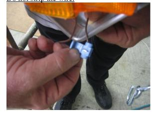
Insert the brown wire from the left (driver's side) running light into the hole in the connector closest to the hinge. This hole does not pass all the way through. The wire should go in about ½".
