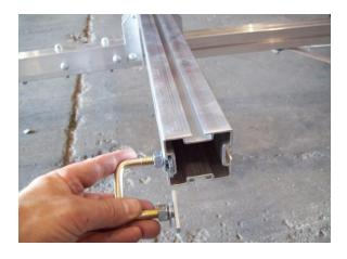
Install 2 clips in the front slot on the front cradle holder.
