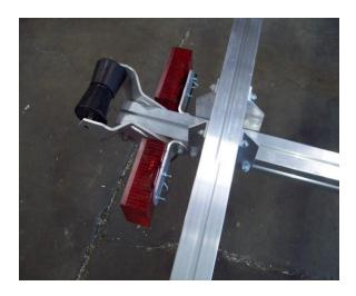
Loosen the tail light brackets, slide the tail lights to the rear as far as possible and slide the rear cradle holder assembly against the tail light brackets. Tighten all nuts.
