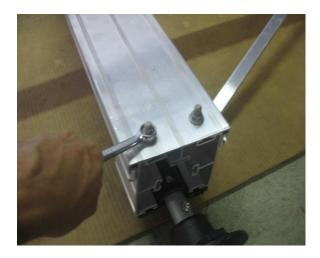
Remove the nuts from the top of the axle assembly.
