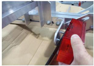
Install the license plate bracket and left tail light onto the tail light bracket.
