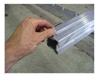
Install (2) 1 1/8" T-bolts into the top slot of the front cradle holder and (1) 1 1/8" T-bolt into the top slot of the rear cradle holder.
