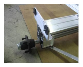
Install the 1" bolts and (2) rubber washers as shown.
