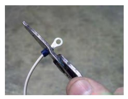
Take the white wire from the harness and strip a ½" of the insulation from the wire. Install ring terminal by crimping it onto the bare wire.
