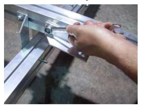
Loosen nuts on other side now and drop the angle brackets down over T-bolts.
