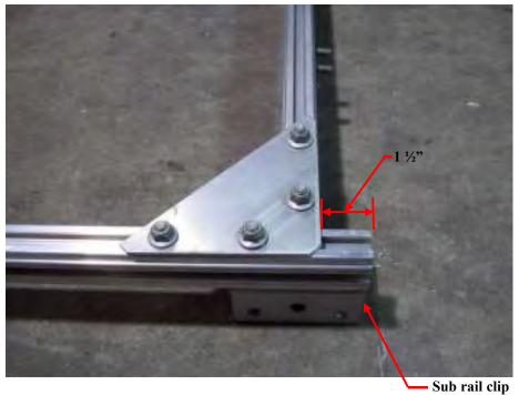
Slide the side rail all the way to the edge of the sub rail clip as shown. The side rail should be about  $1 \frac{1}{2}$  pass the rear cross member when in position.
