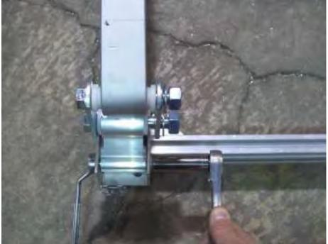
Remove the two bolts from the shackle holder at the rear of the spring and install the shackle holder into the rear sub rail clip, with the nuts toward the inside of the trailer. These nuts can be tightened at this time.
