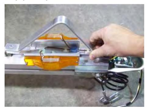
Insert skid with T-bolt into tongue section and over top of the other T-bolt already there.
