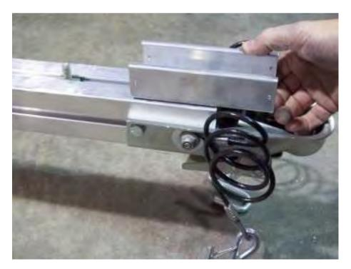
Slide the running light bracket into the slot in the front tongue section.
