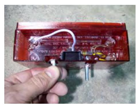
The light with the yellow wires is for the left (drive's side) of the trailer. Slide the carriage bolts into the slots in the back of the tail lights.
