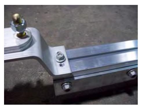
Loosen the T-bolts and nuts on spare tire carrier. Insert into the underside of the front tongue at the rear. Once T-bolts are in channel slide towards the coupler.
