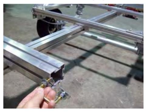
Install 2 clips in the front slot on the front cradle holder.
