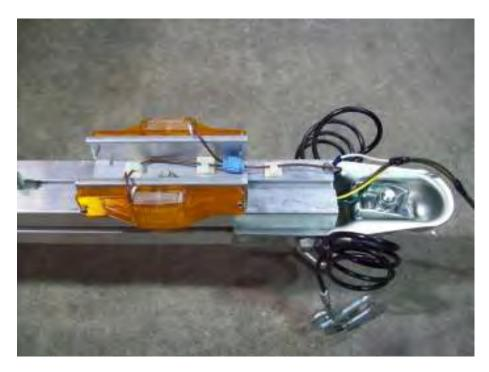
Locate the adhesive backed clamps. Install them as shown and run the brown wire from the running lights through them. Tuck the excess harness inside the tongue.
