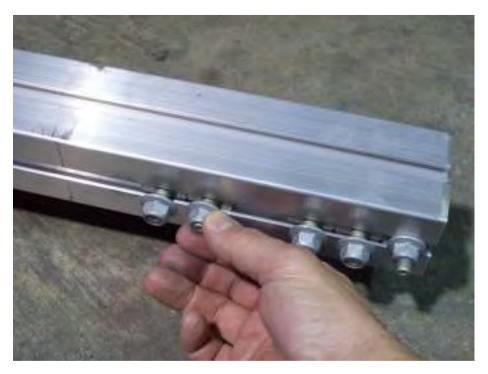
Slide the next two forward facing T-bolt on either side of the rear tongue section to the pencil marks.
