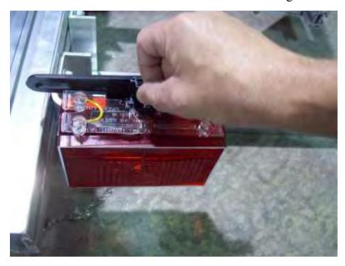
Move the tab toward the rear of the trailer and pull up, releasing the bulb assembly from the light housing.
