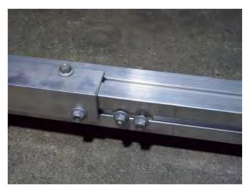
These T-bolts will be used to attach the front cradle holder later.
