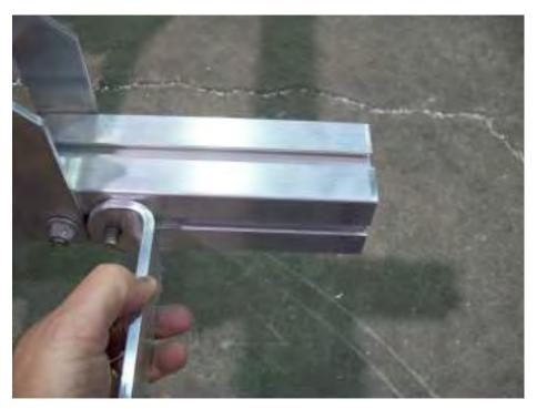
Install taillight brackets over T-bolts and butt up against angle brackets.
