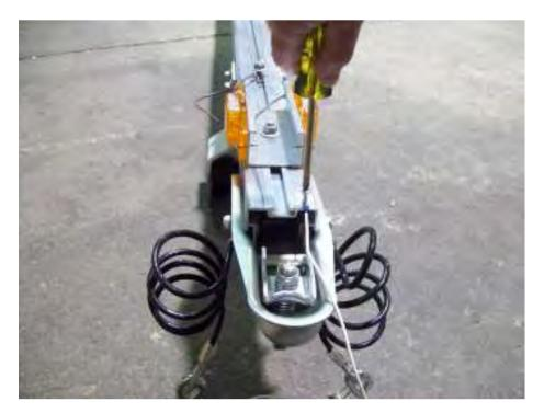
Install Philips screw through the ground wire into the pre-drilled hole located under the tongue just behind the coupler.
