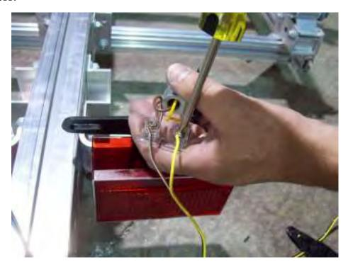
Loosen the retaining screws and install the color matching wires from the harness onto corresponding retaining screws. Tighten screws.
