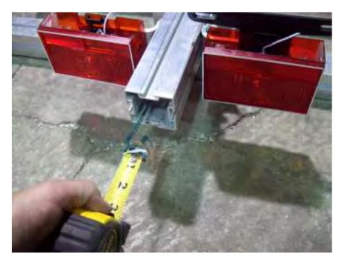
Retract the tape measure until it comes out the back of the tongue with both wires attached.
