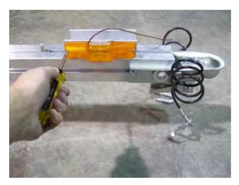
Install the running lights into the pre-drilled holes in the running light bracket using a Philips screwdriver. Be sure the screw is through the ring terminal on the back side of the lights. This will supply a ground to the lights.
