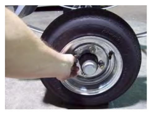
Install the wheels with the valve stems facing out. Install the lug nuts with the tapered side facing the wheel.
