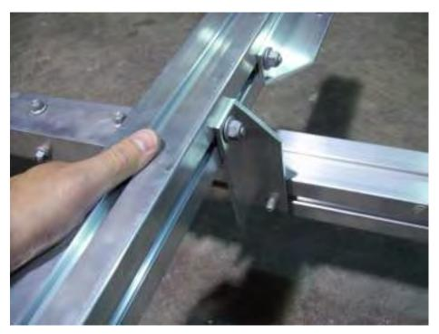
Install angle brackets over T-bolts as shown.
