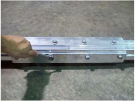
Tighten all 16 nuts, making sure that the tongue sections are as tight as possible to one another. Set the tongue aside.
