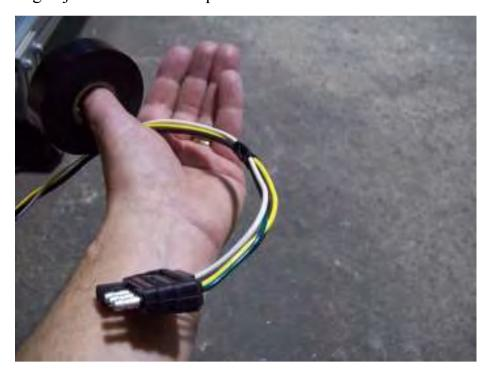
Start taping harness just past the four way connector with electrical tape and work your way down the ground wire to the tongue of the trailer. Usually space the tape about a hands length apart.
