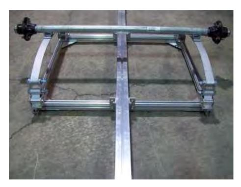
Locate the axle and install it on the springs as shown. Make sure the locating studs on the springs are in the holes on the axle's spring seat. Face the axle's serial plate toward the rear of the trailer to protect it from debris.
