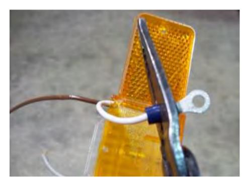
Install the ring terminals by crimping the terminal onto the bare wire.
