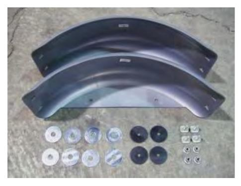
Locate the fenders, 8) large steel washers, 4) rubber washers, 4) 1 1/8" T-bolts and 4) nuts.
