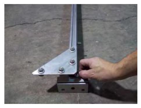
Install 2 T-bolts into the rear side of the rear cross member as shown.
