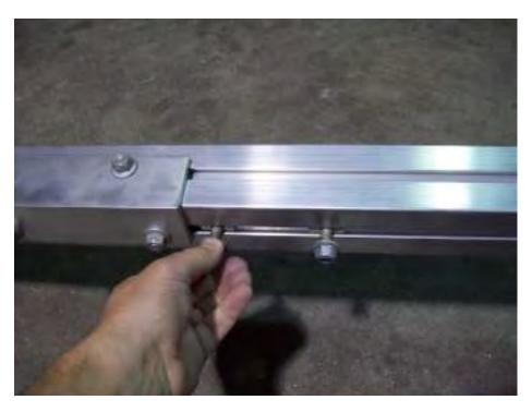
Remove the nuts from the T-bolts next to the splice plates on both sides of the tongue section.
