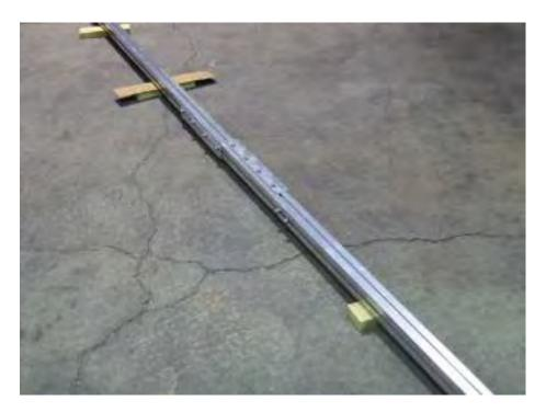
Helpful hint: Place a couple of 2 x 4 under each of the tongue section to make it level. This will help with alignment and sliding the splice plates into position.
