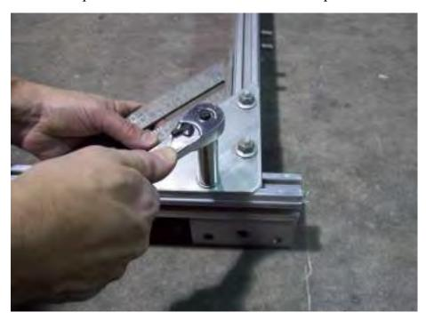
Square up and tighten nuts. Repeat the process for the other side at this point.
