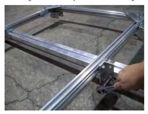
Align the angle brackets inside the pencil marks on the tongue. Re-install nuts and tighten, once in position.
