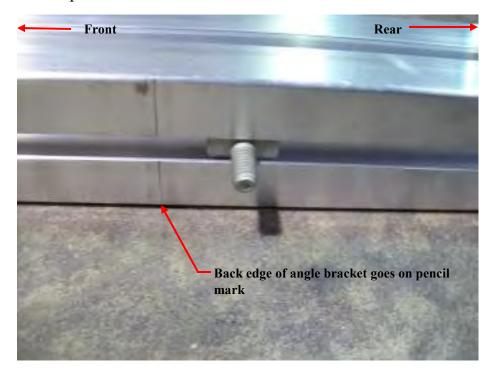
Make sure T-bolts are behind the pencil mark as shown facing the rear of the tongue section.
