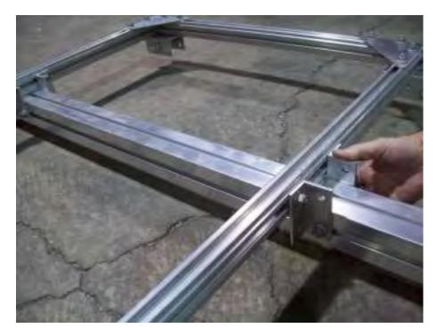
Slide the angle brackets from the right side over and install nuts.
