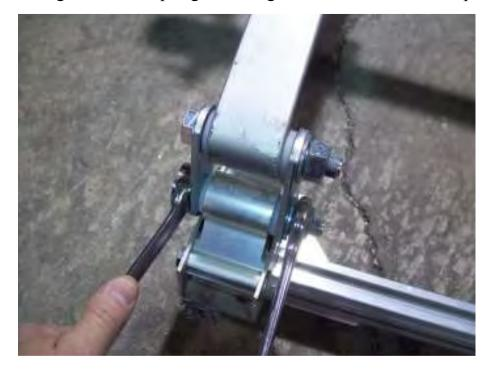
On the rear shackle, do not over tighten as this will not allow the suspension to move properly.
