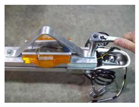
Re-install nut and tighten in position.
