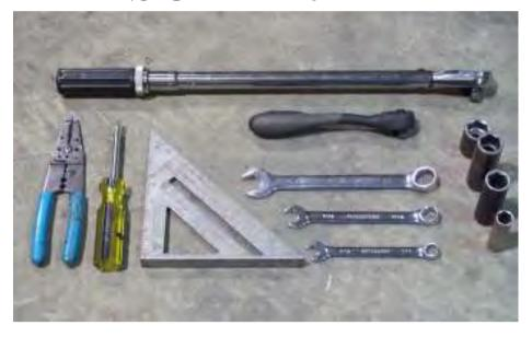
Torque wrench, carpenters square, wire cutters, Phillips screwdriver, 7/16, 9/16, and 3/4" combination wrenches, ratchet, 9/16, 3/4, 13/16", and 7/8" sockets.
