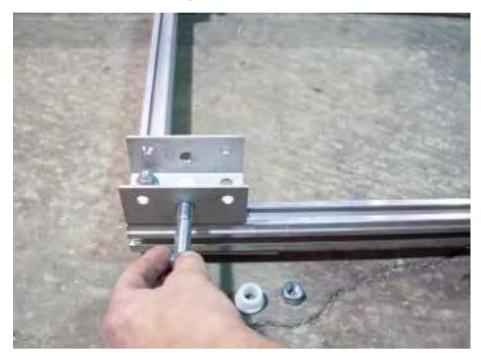
Remove the bolt, bushings and nut from the front sub rail clip.
