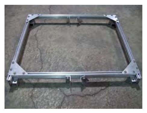
Your frame should look like this, with the angle brackets attached to the rear side of each cross members.
