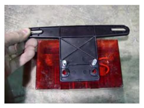
Install the license plate bracket onto the left taillight as shown.
