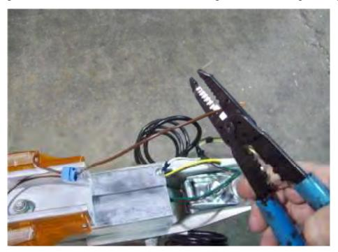
Cut the exposed strands of wire off of the end of the brown wire on the right (passenger side) running light.
