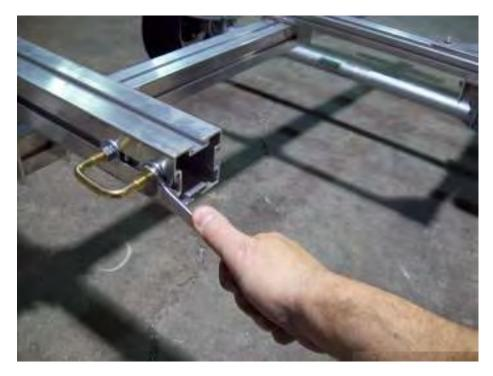
Tighten the nuts. Repeat by installing 2 clips in the rear slot of the rear cradle bracket.
