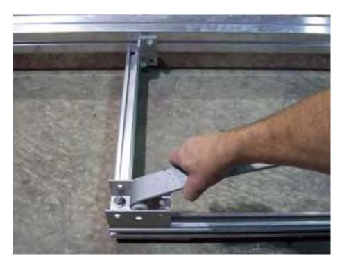
Install bushing into the front leaf spring and insert into the sub rail clip as shown.
