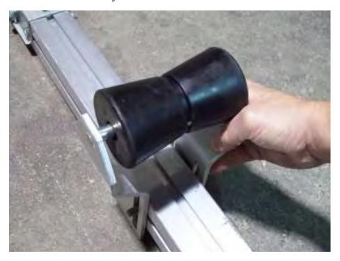
Pull the bracket over top of the other T-bolts to get in place.
