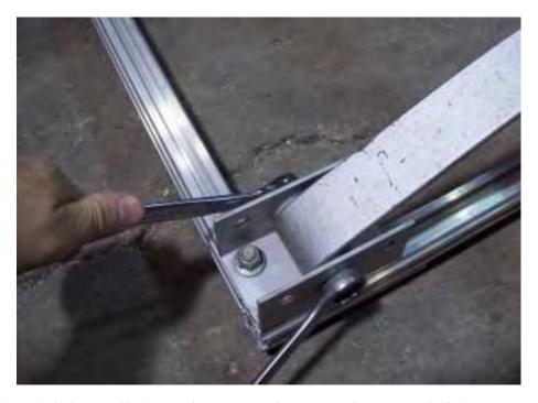
Go back and tighten all the spring mounting nuts that were left loose previously.
