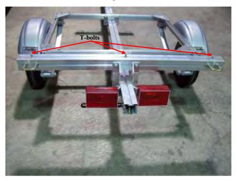
Install three T-bolts in the top of the rear cradle as shown. At this point you should refer to the Hobie instructions for installation of the cradles.
