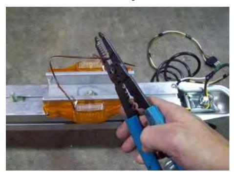
Cut about 2" off the brown wire on the left (driver's side) running light. <u>Do not strip the wire.</u>
