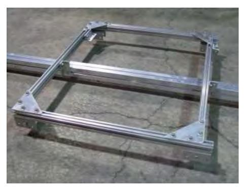
Install angle brackets over top of the T-bolts in the tongue.
