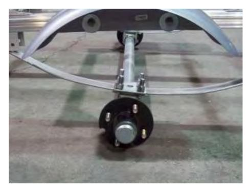
Install the fender, two more steel washers, and nuts, center the fender over the axle and tighten the nuts. Repeat for the other side.
