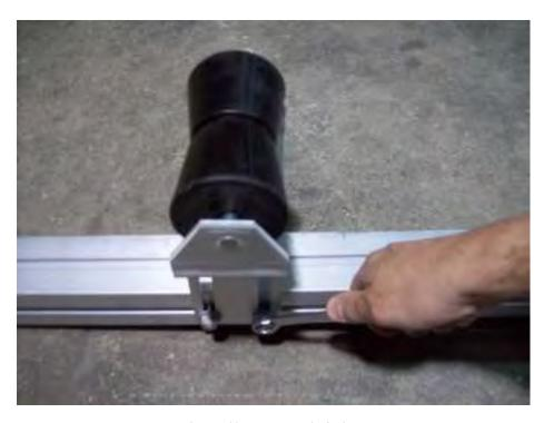
Reinstall nuts and tighten.
