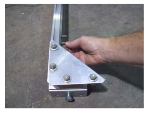
Install 2 T-bolts into the rear side of the front cross member as shown.
