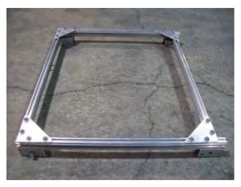
Your frame should look like this. Notice that the side rail extends past the rear cross member. If not assembled properly, the spring assembly will not have enough arch to work correctly.
