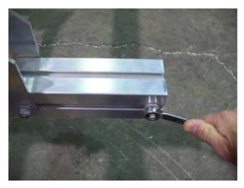
Loosen the last nuts on each side of the tongue section and side them all the way to the angle brackets.
