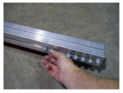
Slide two of the forward facing T-bolts located on either side of the rear tongue section all the way forward to the splice plates.
