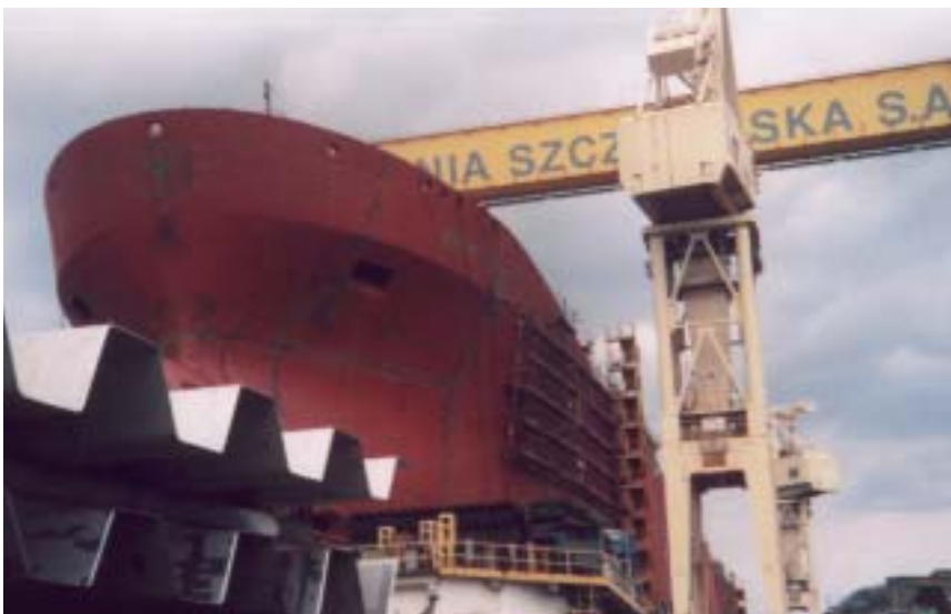
The Bow Star, the second of six 39,500 dwt duplex chemical tankers to be built by Stocznia Szczecinska Nowa.
