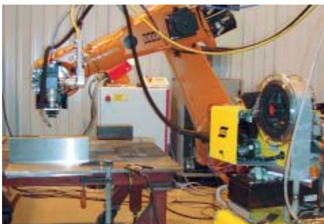
Figure 2 . Laser hybrid welding head installed on a KUKA welding robot. Lappeenranta University of Technology, 2003.
