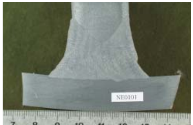
Figure 5. Macro structure of the T-joint taken from a test sample.
