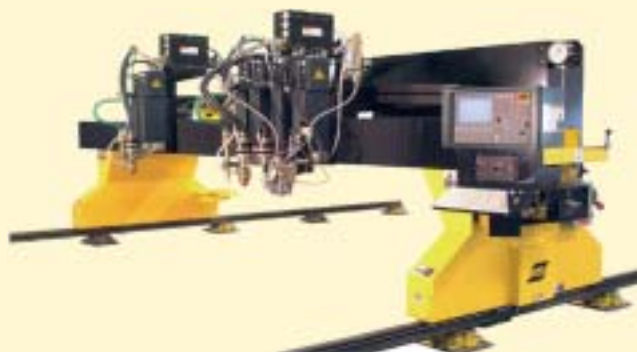
Shown with Waterjet, Plasma Marker, (2) 600 Amp Plasma, and (2) Oxyfuel Stations
