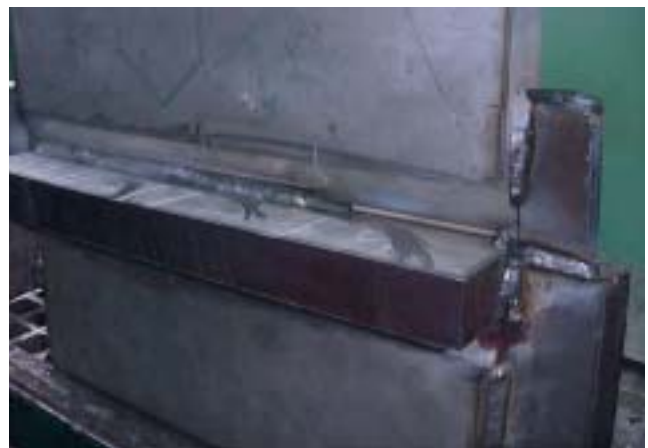
Figure 3. Test coupons welded under full restraint.
