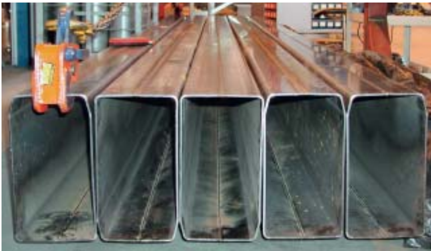
Figure 1. Laser hybrid welded telescopic beams. DinoLift Oy, Finland.
