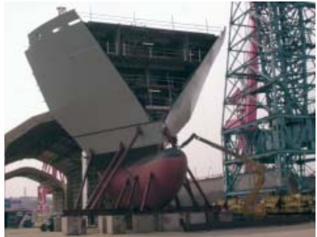
Figure 1. Bow section of second ship ready for transfer to dry dock.
