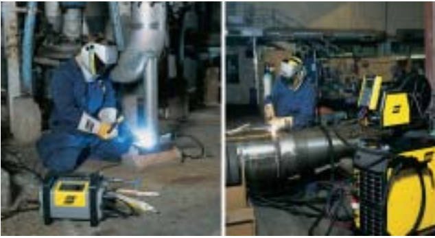
Figure 2. Inverter power sources. Left is an example of low weight and size. Right is inverter based advanced MIG equipment.
