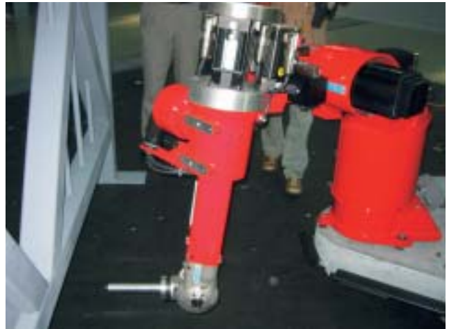
Figure 3. The RTV positioning the robot arm for welding.
