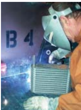
Figure 2. The author welding a thin heat exchanger made of 3xxx series (aluminum/manganese) with pulse spray and 4047 (12% Silicon) filler alloy... a very different welding procedure than that used in fig 1.
