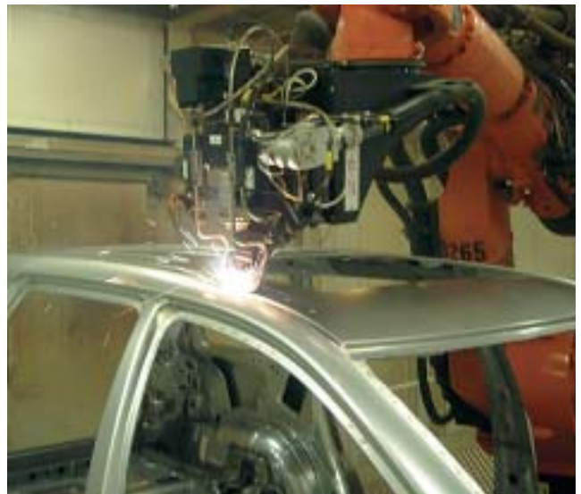
Figure 6. Laser welding of a Volvo XC 90 roof, with pressure roller in front of the laser beam. Permanova Lasersystem AB
