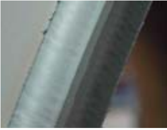
Figure 4. Plasma cut X-bevel. Smooth surface and little dross.
