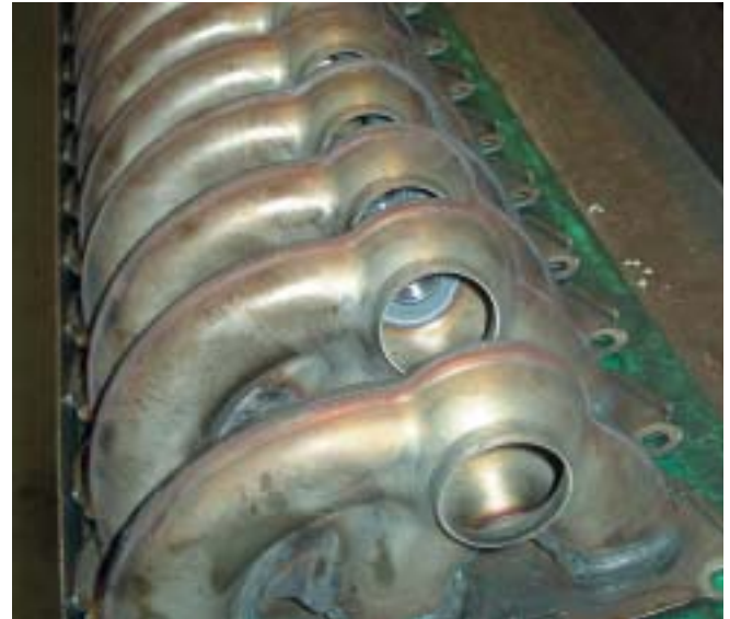
Photo: Benteler, Warburg, Germany. Hot ends of a ferritic stainless steel exhaust system robot welded with OK Autrod 430LNb. This wire belongs to ESAB's new range of matte stainless steel MIG wires with excellent feeding properties and arc stability.
