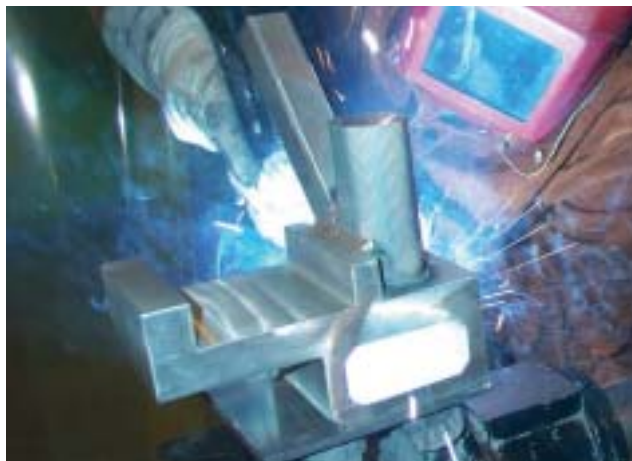
Figure 1. The author MIG welding a thick 6xxx series (Al/Mg/Si) extrusion using a 5356 (5%Mg) filler alloy and high current spray transfer settings.
