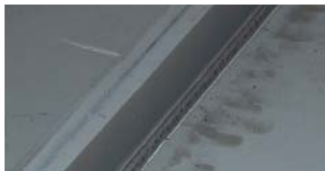
Figure 4. Equal leg length, no porosity, low distortion fillet with Tubrod 14.11.
