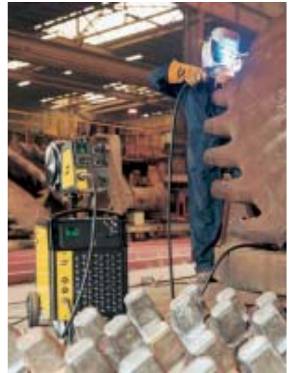
Cover photo courtesy Nista BV, Amsterdam, The Netherlands. MAG repair welding of cutter heads.
