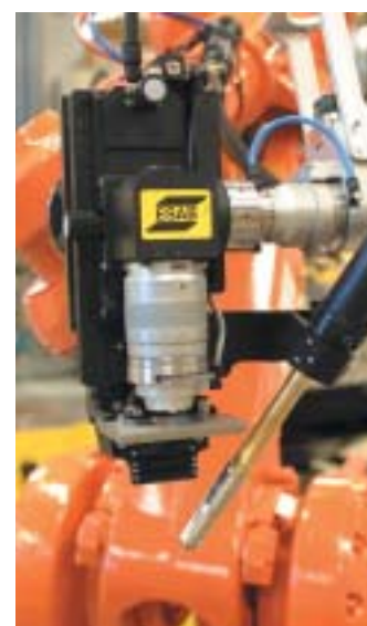
Figure 3. Laser hybrid welding head designed and engineered by ESAB and Permanaova Lasersystem AB.
