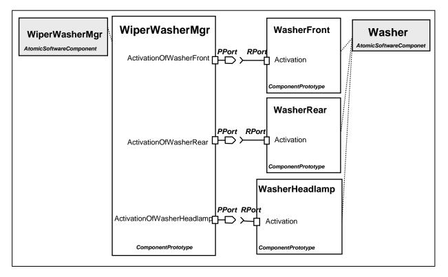
Figure 2: Ports of multiple ComponentPrototypes.
