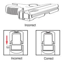
Pull the slide rearward and release it to be sure that the pistol is properly reassembled.
