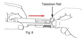
Remove the takedown rail by sliding it off the rear of the slide (Fig. 8).
