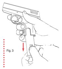
and thereby can create the risk of exploding an unchambered cartridge and possible causing injury. **Visually inspect the barrel chamber to be sure it is empty.**
