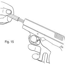
Remove the takedown and assembly tool from the barrel (Fig.15).
