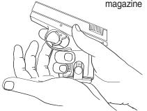
After securely inserting the magazine into the pistol pull the slide fully to the rear. Release the slide and allow it to move all the way forward. This strips a cartridge from the magazine and seats it in the chamber of the barrel, making the pistol ready to fire. **The pistol can now be fired by pulling the trigger.**
