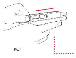
Empty the magazine by holding it with the bullet end of the cartridge pointing away from you and pressing each cartridge forward and out of the magazine.
