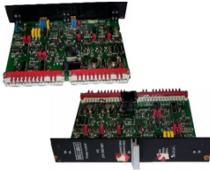
Main control PCBs for Crane systems
