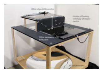
Figure 11. A tabletop Floating Switching Dual Layer Display using a 36" diameter, 15" FL concave mirror and two 23-inch 120Hz monitors. The mirror relays an image of the relayed monitor so it floats above the transparent monitor.
