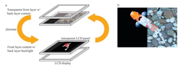
Figure 3a. A Switching Dual Layer Display alternates between front layer content with back layer backlight, and clear front layer with back layer content. b. Stacked LCDs combine additively. Front layer content appears over dark background content (left), and front layer content appears semi-transparent and low-contrast over bright background content (right).
