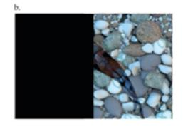
Figure 1a. A basic dual layer display using a transparent LCD panel stacked and spaced over a LCD monitor. b. Stacked LCDs combine multiplicatively. Front layer content does not appear over dark background content (left), and front layer content appears dark, low-contrast, an semi-transparent over bright background content (right).
