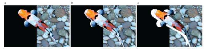
Figure 2a.Pure Depth's Multilayer Display makes the front layer content visible and apparently opaque (when viewed onaxis) by aligning front layer content with a matching white silhouette on the back layer. b. A halo appears when viewed slightly off-axis due to parallax between layers. c. White silhouette apparent when viewed off-axis.
