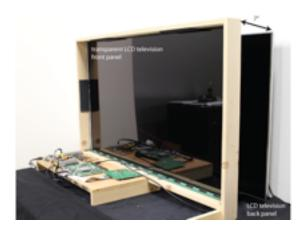
Figure 6. A Switching Dual Layer Display using two stacked and spaced 55" LCD televisions.
