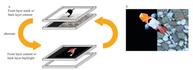
Figure 4a. A Switching Dual Layer Display with a Dynamic Mask alternates between front layer content with back layer backlight, and front layer mask with back layer content. b. Front layer is independent of back layer content. Front content appears over dark background content (left), and front layer content appears opaque and high-contrast over bright background content (right).
