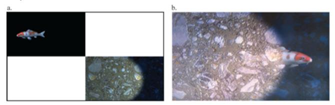
Figure 9a.Double-wide over-under image format for switching Dual Layer Display with Mask with front layer content (upper left), front mask (lower left), and background content (lower right). Left frames displayed on front transparent LCD panel; right frames displayed on rear LCD monitor. b.Image from the Switching Dual Layer Display with Mask, alternating
