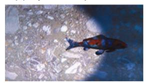
Figure 7. Image from the Switching Dual Layer Display acting as a basic Dual Layer Display (without switching), where front and back content are multiplicatively blended. Front layer content does not appear over dark background content, and appears semi-transparent, dark and low contrast over bright background content.
