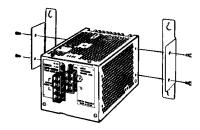
Note: Mount the Unit 21.6 mm away from the mounting surface in order to provide air ventilation on the rear side.
