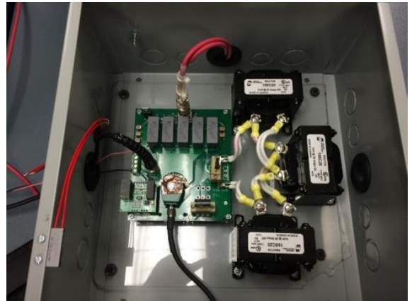
Fig. 5. Photograph of DPTC used for switching stress of the v-GaN diodes.
