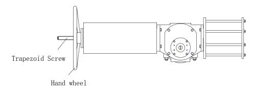
SY01F14 & SY01F16 after manual operation, screw out the trapezoid screw when it change to auto-operation way, to ensure the auto-operation smoothly realized. Avoid to screw out integral trapezoid screw, the valve open & close position will be influenced if the screwing is not in place.
