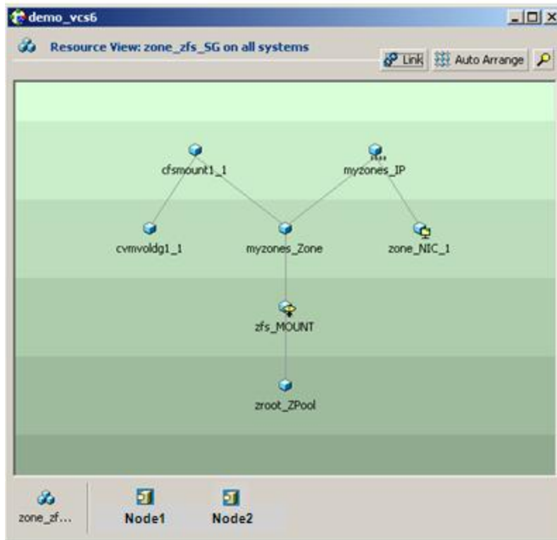
Figure - 19 ZFS and Cluster File System Coexistence
