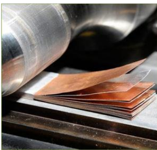
Figure 42 Sheet lamination at work. Sheets are fused together using ultrasounds. Image credit: Loughborough University
