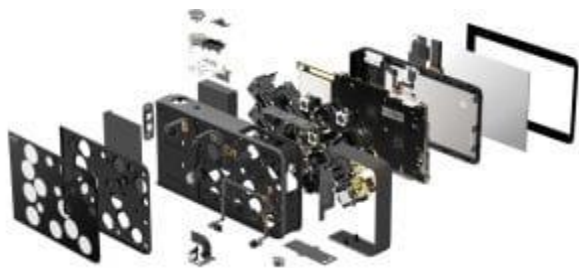
Figure 74. The L16 has 16 lenses, each time you take a photo you are using several of them, and software takes care of fusing the individual lens output into a single photo. Image credit: Macfilos
