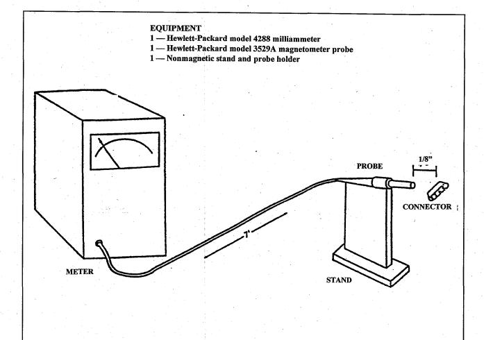
Figure 1. Residual-Magnetism Test Arrangement
