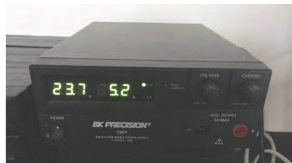
Fig 2: Adjustable digital DC power supply to the electrical heater.
