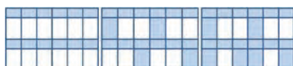
Fig 4: Schematic examples of elevations designed by combination of the vision/spandrel units. From left to right: classic elevation with 88% vision, 60% vision, 44% vision.
