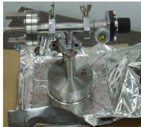
Fig 1: A photograph of an mVIP system connected to the envelope of a 25cmX25cm VIP. The system contains Spinning Rotor Gauge (SRG) for measuring the internal pressure, as well as extra an opening for VIP evacuation, He leak checking and RGA measurements.
