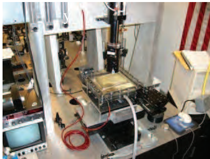
Fig 1: Laser setup for 25 cm samples. Red tube is for Argon gas (flows below & above stainless steel foil). Clear tube is for vacuum.
