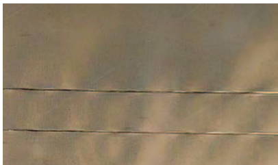
Fig 2: Laser welded stainless steel, weld width is ~0.5 mm.
