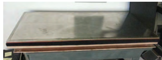
Fig 1: Picture of the hot test plate that can test 6 sample panels at one time.
