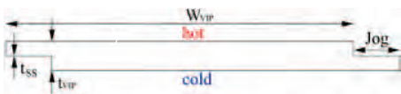
Fig 3: A VIP with width W_{VIP} and thickness t_{VIP} , can minimize thermal edge losses with the indicated Jog.
