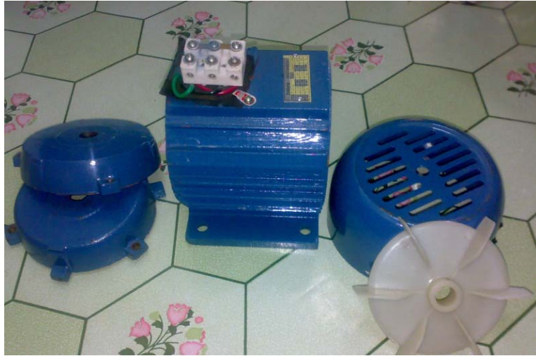
Figure 3.9: Type of enclosure used
