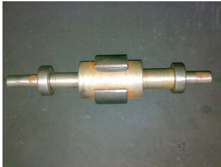
Figure 3.8: Mounted magnet on the rotor shaft
