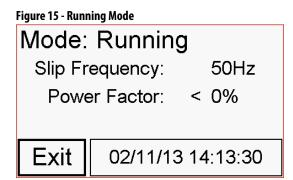
In the *Running* mode, the slip frequency and power factory is displayed. During normal operation, the slip frequency is 0 Hz, and power factor is approximately 100% for unity.
