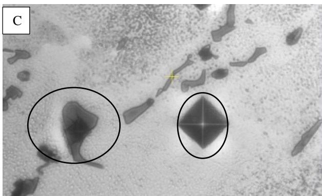
Figure 4-8: A. Chinese script and B. thin plates of \beta -Fe intermetallic, C. microhardness of the \beta -Fe intermetallic and the matrix
