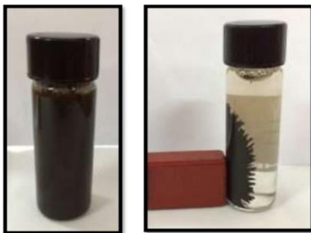
Figure 20. The separation and redispersion of a solution of GO-200 nm / Fe 3 O 4 in the absence (left) and presence of an external magnetic field (right) .
