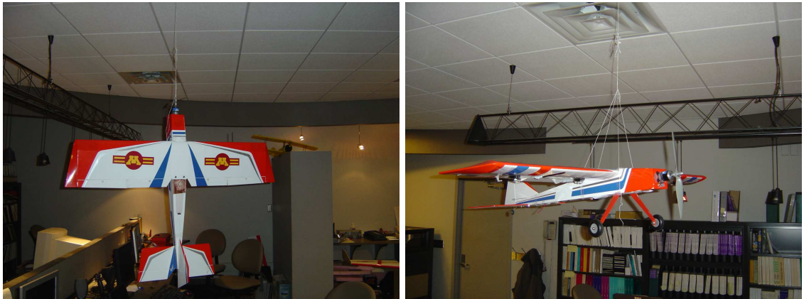
(a) Pendulum swing setup for I_{zz} determination (b) Pendulum swing setup for I_{xx} and I_{yy} determination
