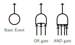
Each gate can have multiple inputs, some of which are "negated," but only one output.
