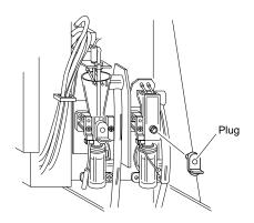
**Figure 4-7-11: Removing the Plug**
