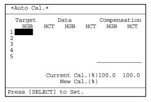
Figure 6-2-4: HGB/HCT Automatic Calibration Screen
