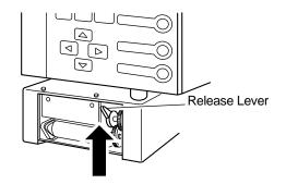
Figure A-6-1: Releasing the Lever
