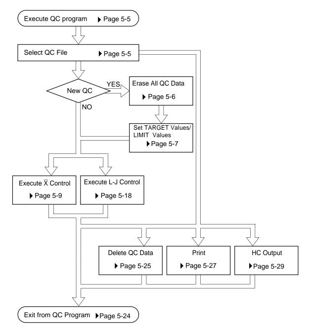
Figure 5-2-1: QC Analysis Procedure Flow Chart
