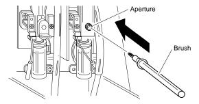
Figure 4-7-12: Cleaning the Aperture
