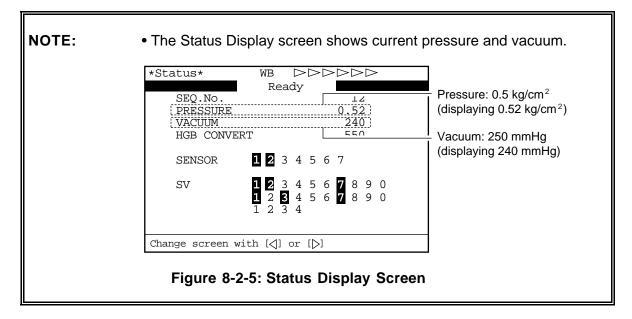
(6) Adjust the pressure and vacuum by following the procedures given on the next page and later.
