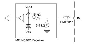
Figure B-1-2: Interface Input Circuit
