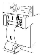
Figure A-6-3: Securing the Release Lever
