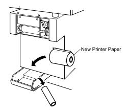
Figure 4-8-5: Mounting a New Printer Paper
