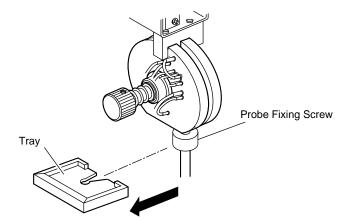
Figure 4-6-3: Removing the Tray
