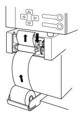
Figure 4-8-6: Securing the Release Lever
