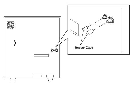
Figure A-4-4: Removing the Rubber Caps
