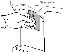
Figure 4-5-3: Pressing the Start Switch
