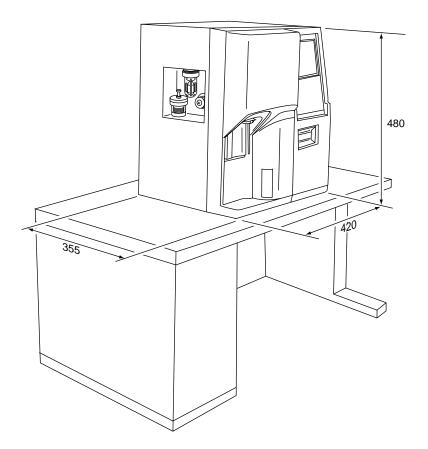
**Figure A-3-1: Instrument Dimensions**
