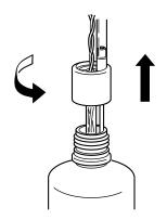
Figure 4-8-1: Pulling Out the Cubitainer Spout Set
