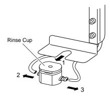
Figure 4-7-4: Removing the Rinse Cup
