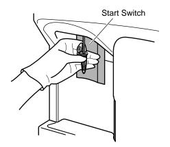
Figure 2-4-13: Pressing the Start Switch
