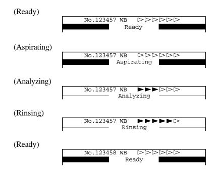
Figure 2-4-7: LCD Screen (in WB Mode)
