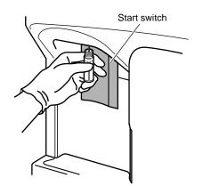
Figure 5-2-12: Pressing the Start Switch
