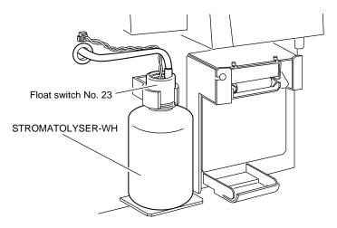
Figure A-5-4: Installing the STROMATOLYSER-WH
