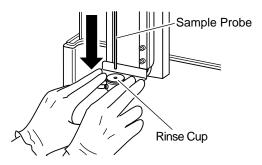
Figure 4-7-3: Pushing Down the Rinse Cup
