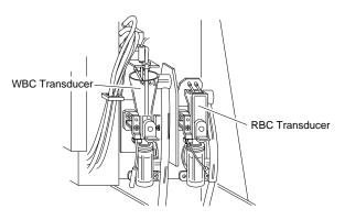
Figure 4-7-10: Checking the WBC/RBC Transducer
