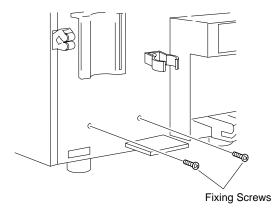
**Figure A-4-3: Removing the Screws**
