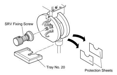
Figure A-4-2: Removing the Protection Sheets
