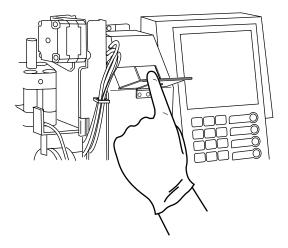
Figure 4-5-7: Opening the Transducer Cover
