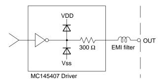
Figure B-1-1: Interface Output Circuit
