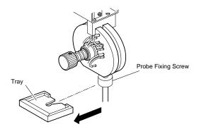
Figure 4-4-1: Removing the SRV Tray
