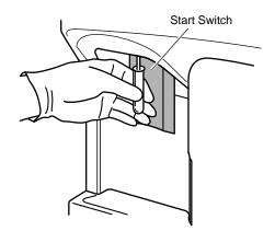
Figure 2-4-6: Pressing the Start Switch
