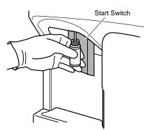
Figure 4-3-2: Pressing the Start Switch
