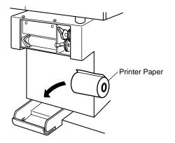
Figure A-6-2: Mounting a Printer Paper
