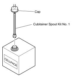
Figure A-5-1: Setting the Cubitainer Spout Kit
