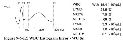
17) 7 The particle count equal to or less than LD is higher than the range. PLT is flagged with AG and other parameters are not flagged.
