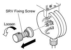
Figure 4-6-5: Removing the SRV Fixing Screw
