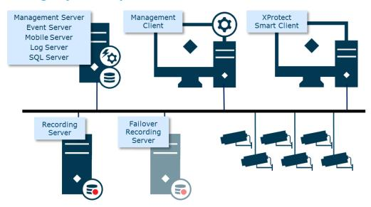
With this design the recording server is installed on a dedicated server to ensure optimal performance. To provide live and recording capabilities in scenarios where the recording server has failed or is stopped for maintenance, a failover recording server can be added.
