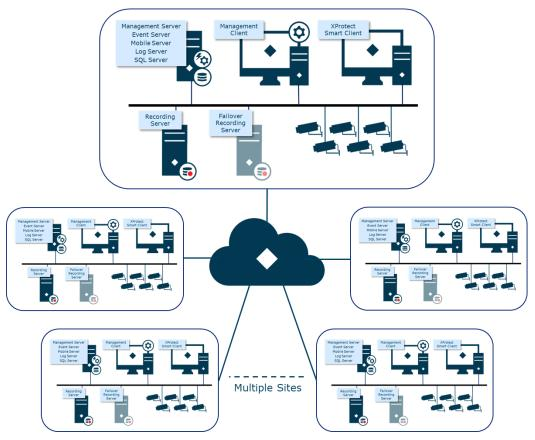
In a geographically distributed VMS system, where the network connection is stable and where users must access video locally on each of the remote sites, it is recommended to design the system using Milestone Federated Architecture.
