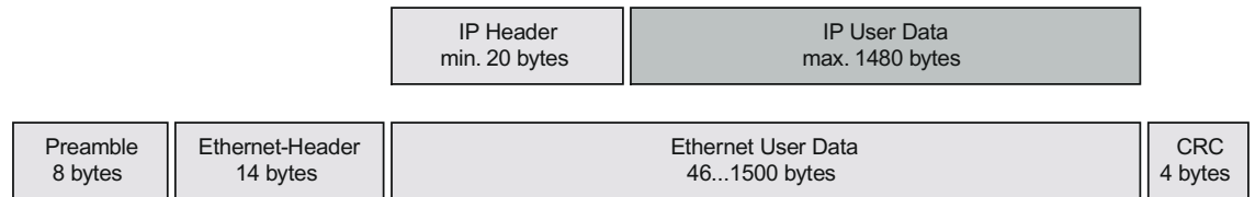
Figure 1-5: IP datagram in the Ethernet frame
