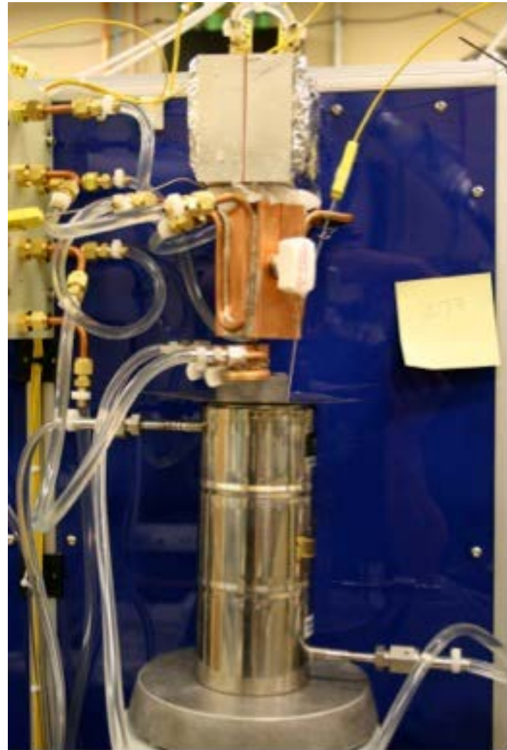
NREL's Sitaram PCTPro System with Temperature Stability Improvements to Measure Hydrogen Isotherms
