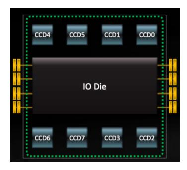
A Rome processor supports 8 memory controllers. Each memory controller supports 2 DIMMs (3200 MHz DDR4), for the maximum memory bandwidth of 409.6 GB/s per socket.
