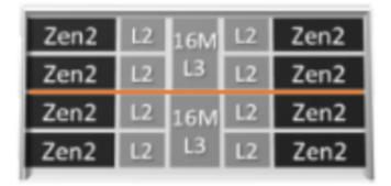
The EPYC 7742 processor has eight CCDs for a total of 64 cores, and one IOD per socket, as shown below.
