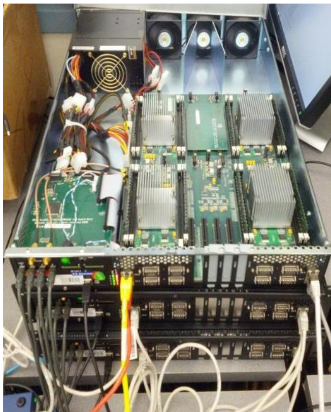
Figure 2.1. BEE3 emulation system using Virtex-5 FPGAs.
