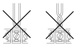
Figure 15: Improper termination
