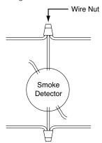
Figure 17: Pigtail Connections - Incorrect Wiring Method
