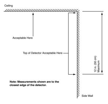
Figure 18: Wall Mounted Detector - Placement
