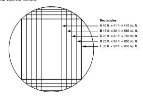
Figure 20: Detector Coverage Patterns
