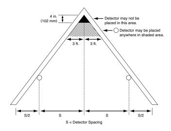
Figure 22: Detector Spacing Layout - Sloped Ceilings (peaked type)
