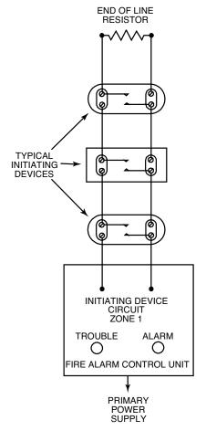
Figure 10: 2-Wire Detector Class B Circuit
