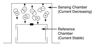
Figure 5: Dual Chamber with Particles of Combustion
