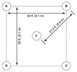
Figure 19: Typical Detector Spacing
