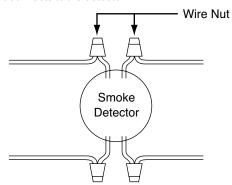
Figure 16: Pigtail Connections - Correct Wiring Method
