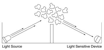
Figure 7: Light Scattering Detector with Smoke
