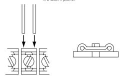
Figure 14: Proper termination
