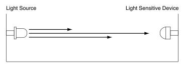
Figure 8: Light Obscuration Detector
