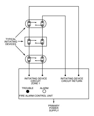
Figure 11: 2-Wire Detectors - Style D (Class A) Circuit
