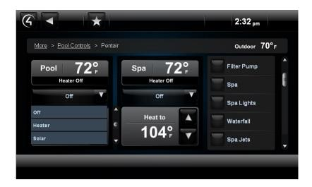
**Note**: Jandy settings have three (3) states: Off (Black), Enable (unless pump is running), and Active (heat is activated). Pentair has two (2) settings: Off and On. See your manufacturer's documentation for details.
