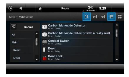
To sort by driver type (sprinkler, lock, and so on) select the icon to the right of AZ (see below). To sort the list, select the icon to the left of the List icon. This list indicates which contact or relay was last changed (by time). **Example**: If you just opened the door, it would appear at the top of the list.
