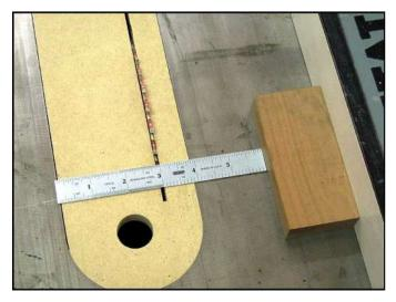
For the first cross cut method, let's cut that 1/4" x 3/8" stock we ripped last time into 3" lengths. Set a nice, clean, squared block of wood against the fence. Set the fence for 3" from the blade to the block.
