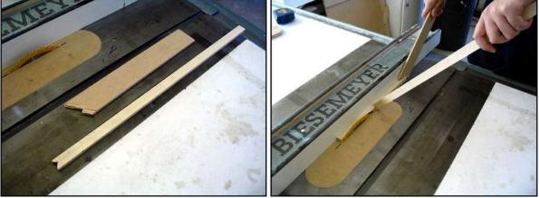
The short stick is for pushing stock through the blade. The longer stick has a notch to help keep stock up against the fence. Here is how they work: Note how chewed up the shorter push stick is. If you don't use a push stick, that's what happens to your fingers. As the sticks wear out replace them. Push sticks are fine to rip bigger lumber, but they are not safe enough to rip thin strips, while cutting scale lumber you'll probably never use a push stick. I don't.
