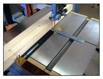
For a rip fence, use any nice straight length of board. Use the setting on the adjustable bevel to set the fence while measuring the thickness of the cut you want from the blade.
