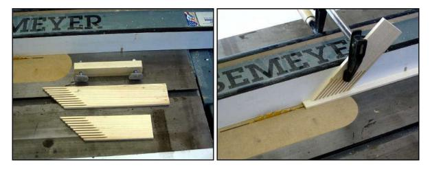
That leaves the longer feather board, which gets clamped to the surface of the saw table; its job is to hold the stock against the surface of the rip fence. The hold down clamp is made from a block of wood, two standard toilet bolts, two washers, and either two wing or hex nuts. The bolt heads are cut to fit the "T" slot on the saw table. Here's how the feather board clamps to the table. Just a heads-up tip, not all table saws have T-slot miter gauge slots.
