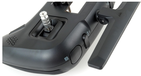
Rocker switch, power button, ports, and speaker
