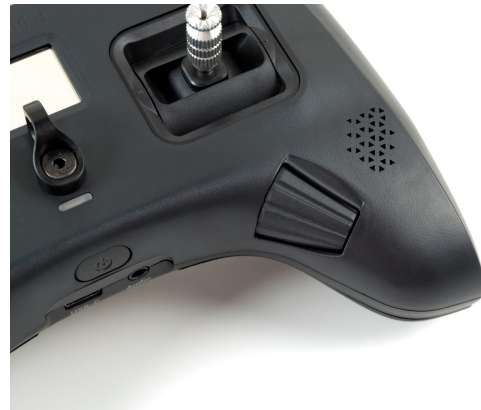
Rocker switch, power button, ports, and speaker
