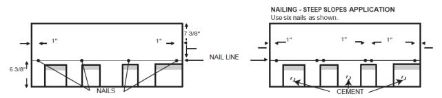
PROPER APPLICATION REQUIRES THAT THE NAILS PENETRATE BOTH THE OVERLAY AND UNDERLAY PORTIONS OF THE SHINGLE
