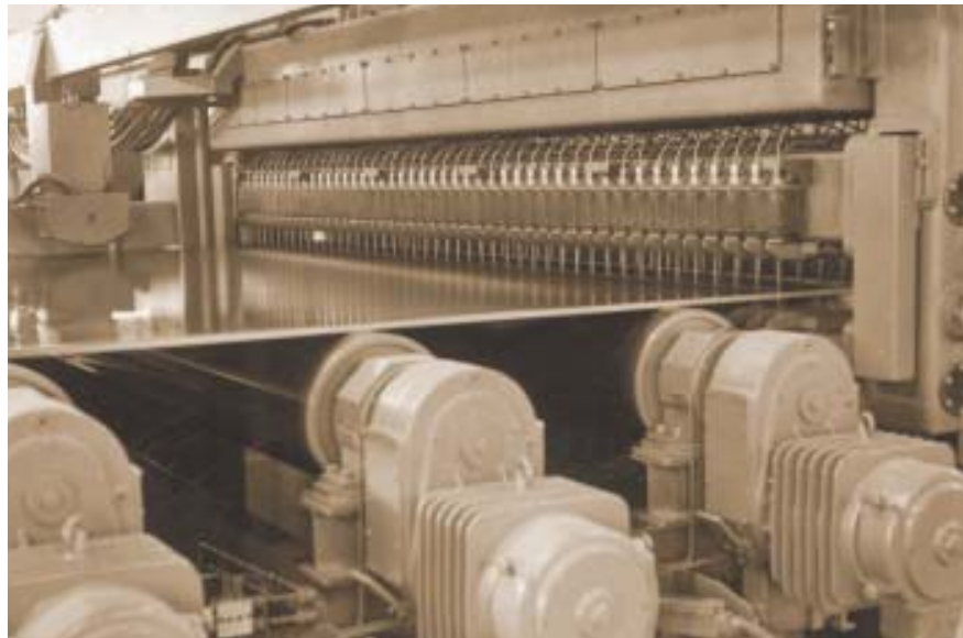
top: Mechanized weld testing using USIP below: Heavy plate testing using free water jets
