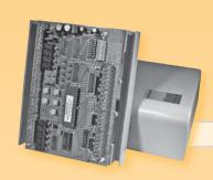
Zone Control Panels are compatible with most conventional, heat pump, and geothermal multi-stage systems. The solid state circuitry incorporates optional features such as: outdoor air temperature sensing, automatic heat/cool changeover, purge cycle and has built in diagnostics.
