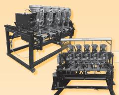
FGMH for welded insulation fastening and HSMH - High Speed Multihead Pinspotter® capable of welding up to 2 inch pins on 16 gauge material as close as 6 inch centers at speeds of 50+ feet per minute.
