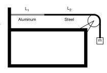
wire by an external source of variable frequency; a node is located at the pulley. (a) Find the lowest frequency that generates a standing wave having the joint as one of the nodes. (b) How many nodes are observed at this frequency?
