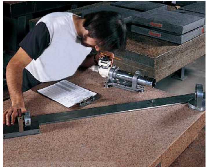
Inspecting a granite plate with an autocollimator.
