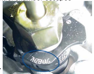
Each Injector has a UNIQUE calibration code etched on the electrical connector.
