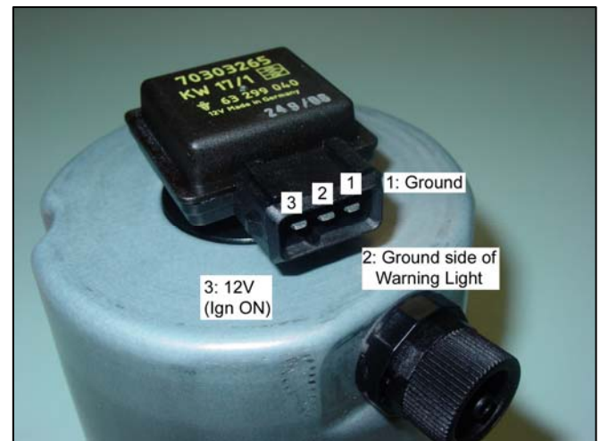
Filter & Sensor are 1 complete assembly. They are NOT separate parts.
